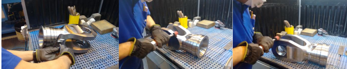
Figure 5 Assembly and auxiliary operation of the main landing gear retraction actuator - Examples of manual deburring process
